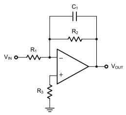
Figure 4-2 Low Pass Active Filter
