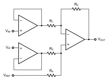
Figure 4-3 Instrument Amplifier
