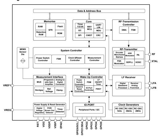
Figure 5-1 Block Diagram
