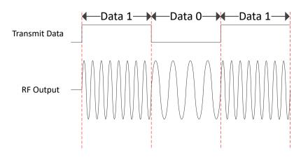
Figure 5-9 FSK modulation
