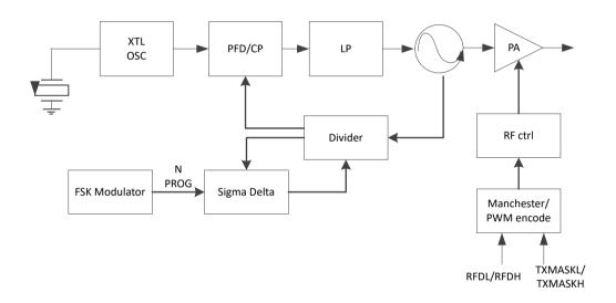
Figure 5-6 RF1 transmitter block
