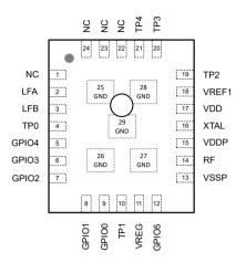
Figure 2-1 Pin Configuration(Top View)
