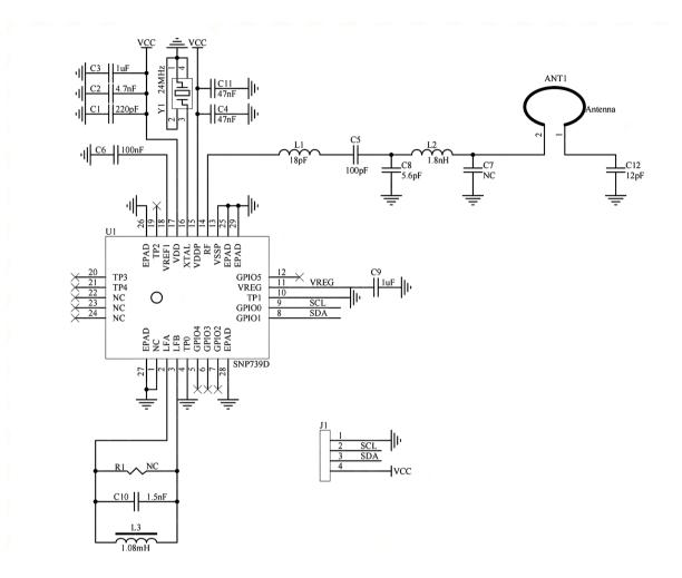
Figure 6-1 Application Circuit
