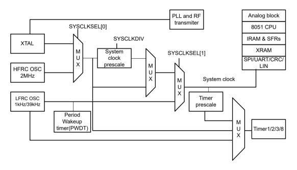
Figure 5-3 Clock distribution diagram.
