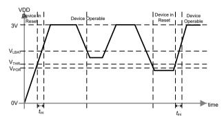
Figure 5-2 Power-On and Under-Voltage Reset Behavior
