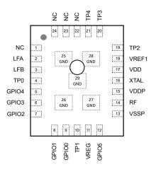
Figure 2-1 Pin Configuration(Top View)
