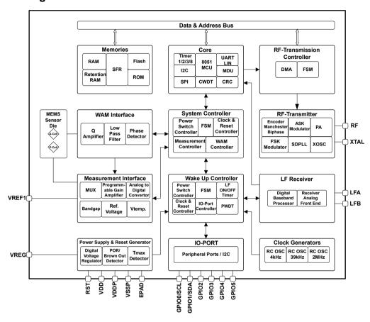
Figure 5-1 Block Diagram
