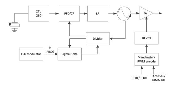
Figure 5-6 RF1 transmitter block
