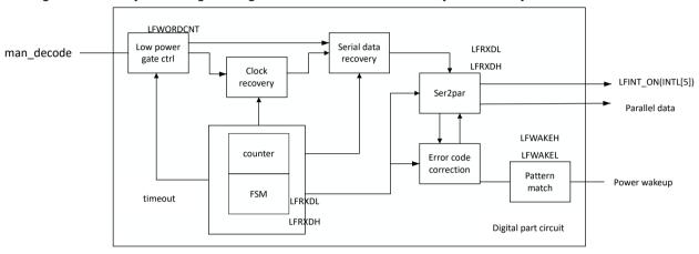
Figure 5-11 LF digital baseband block diagram
