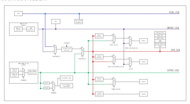
Figure 5-3 Clock distribution diagram.
