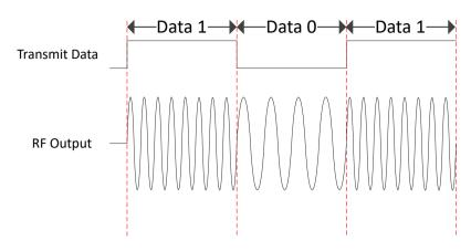
Figure 5-9 FSK modulation
