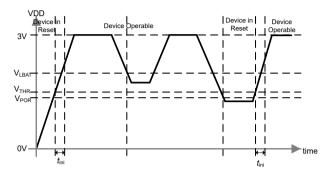
Figure 5-2 Power-On and Under-Voltage Reset Behavior
