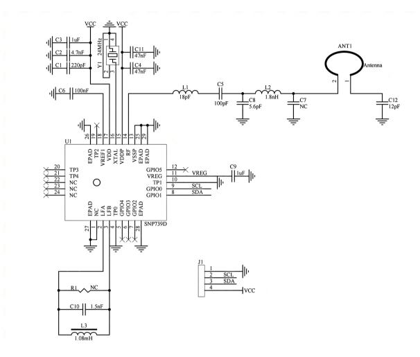
Figure 6-1 Application Circuit
