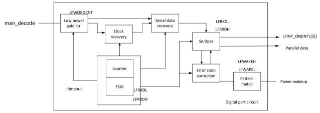
Figure 5-12 LF digital baseband block diagram
