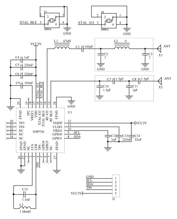
Figure 6-1 Application Circuit
