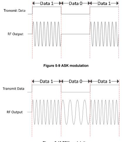
Figure 5-10 FSK modulation
