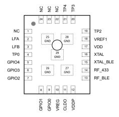
Figure 2-1 Pin Configuration(Top View)
