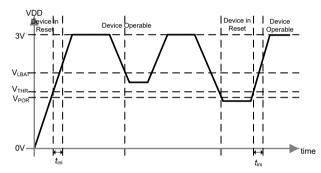
Figure 5-2 Power-On and Under-Voltage Reset Behavior
